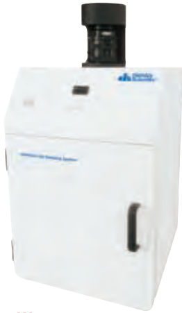
“MaXidoc™ G2” Gel Imaging System, Built-in Transilluminator
