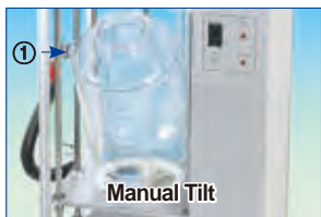
(A) AutoLifting & Manual Tilt Reactor Set, -80°C+260°C
