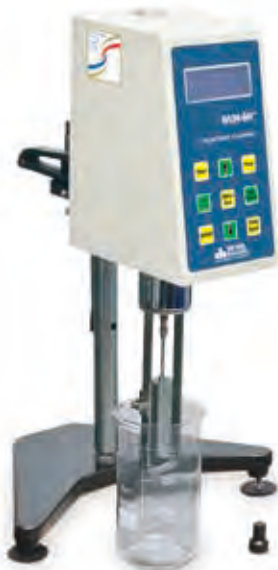
Multi-speed Rotary Viscometer Full Set "WVM"
