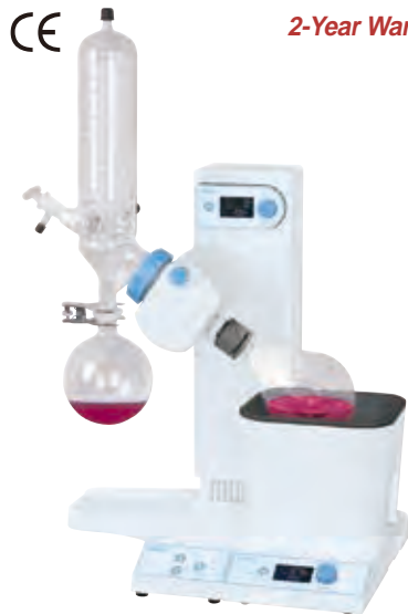
Premium Rotary Evaporator, with 2.5Lit Oil Bath(Included), for 0.1~2Lit Evaporating Flask
