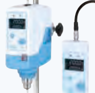
Overhead, Hi-torque ~200,000mPas
