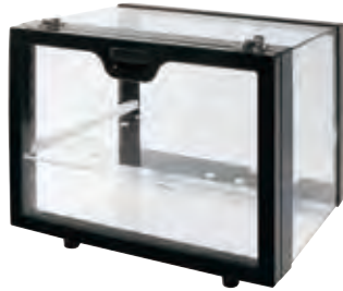
General Purpose Desiccator "DeLL", 33Lit
