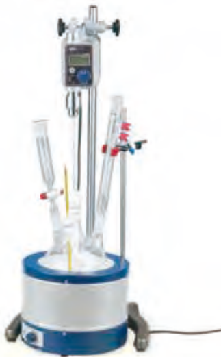
(1) Basic-type Flask Mantle with Controller
