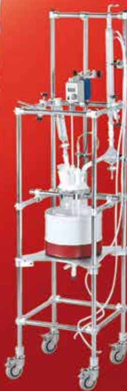
2~50 Lit. H.Mantle-Model IV Single-Wall Vessel Good for Simply Economic Operation
