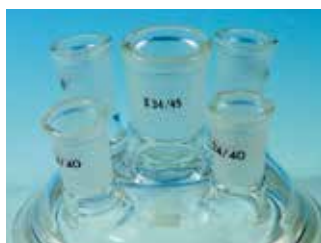
(6) 5-Neck, Tall-form 45° DN flange Lids Center : ₩ 14/23, 24/40, or 34/45 3× 15° angled & 1× Vertical Side-neck
